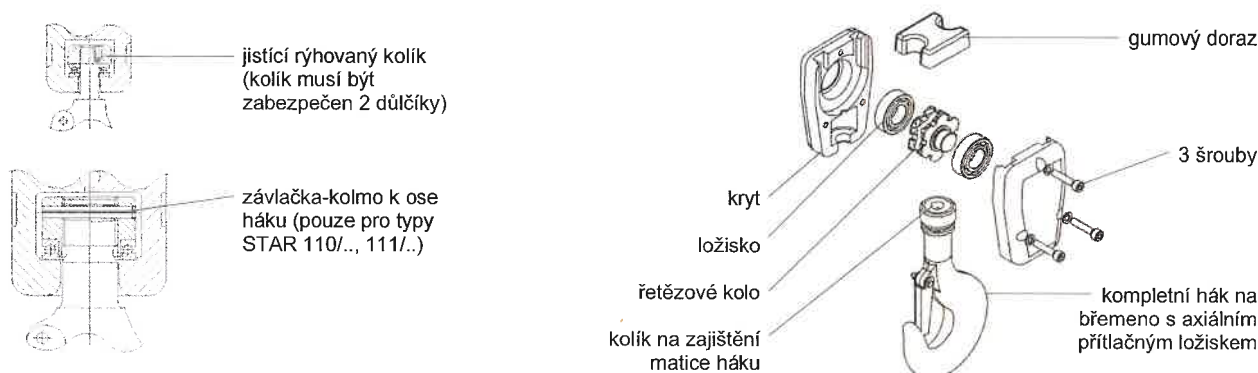
Obr 5: detail kladnice
